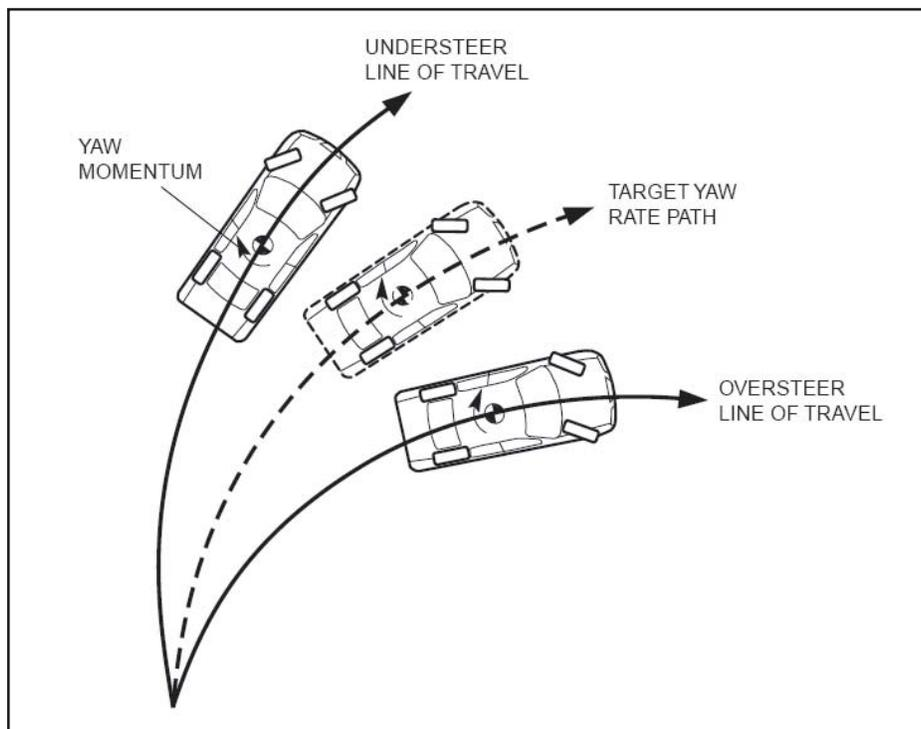
Direction of travel is determined by inputs from the steering angle sensor and the combined sensor. The combined sensor measures yaw angle, and forward and lateral G-forces.
