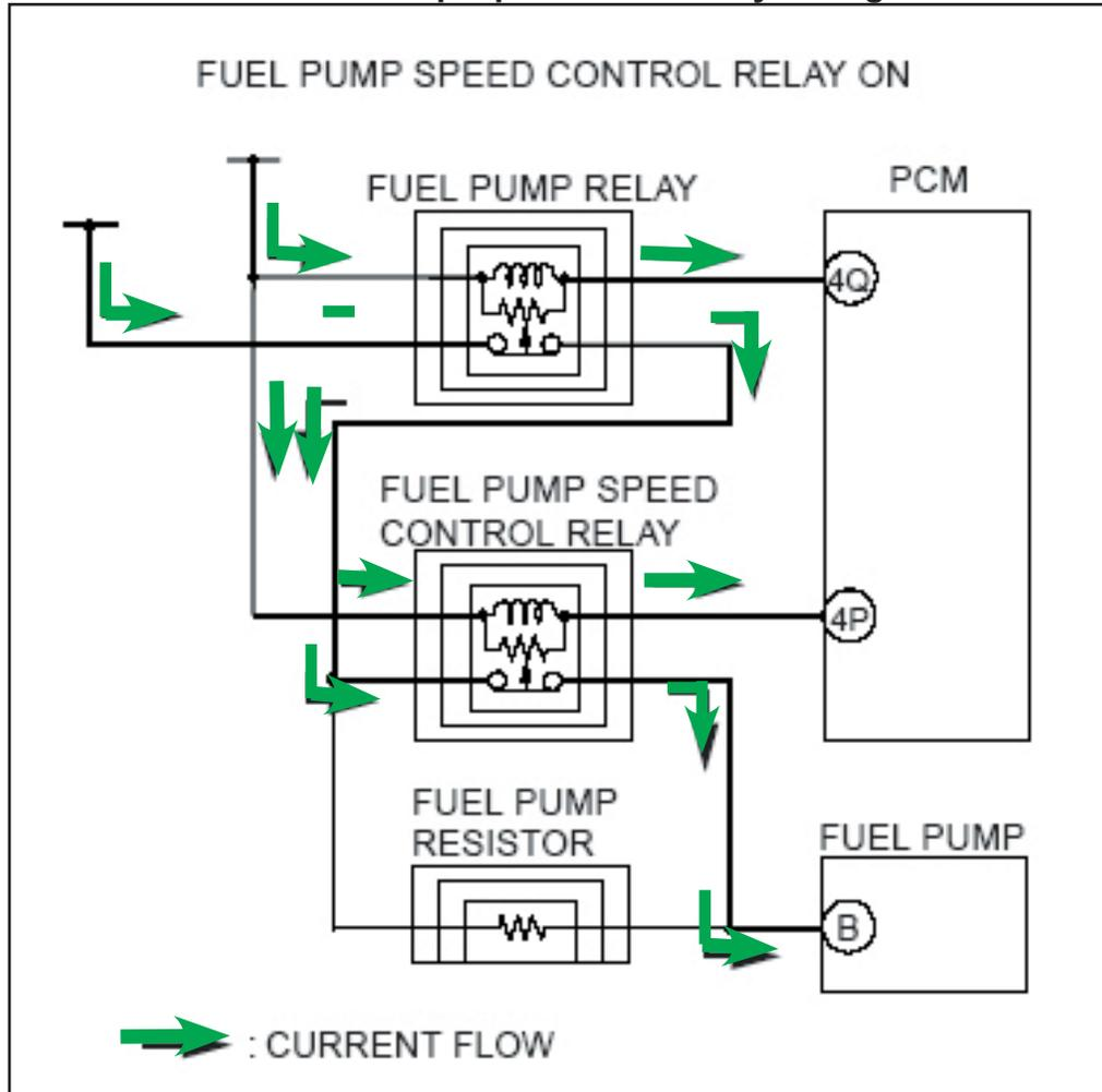
Fuel pressure is inspected in the traditional manner in the engine compartment before the high pressure pump and should be approximately 65 psi. You can also use WDS to monitor the high pressure fuel rail pressure sensor before the engine is cranked. Key on engine off, the in-tank fuel pump pressure is displayed. The fuel pump resistor is located in front of the drivers side strut tower.
