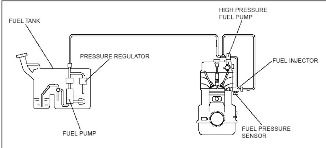
Fuel pressure from the in-tank pump is controlled at two voltages; low voltage for idle when less fuel volume is required and high voltage for high volume required during higher engine speeds. Voltage and volume change but pressure is constant.
