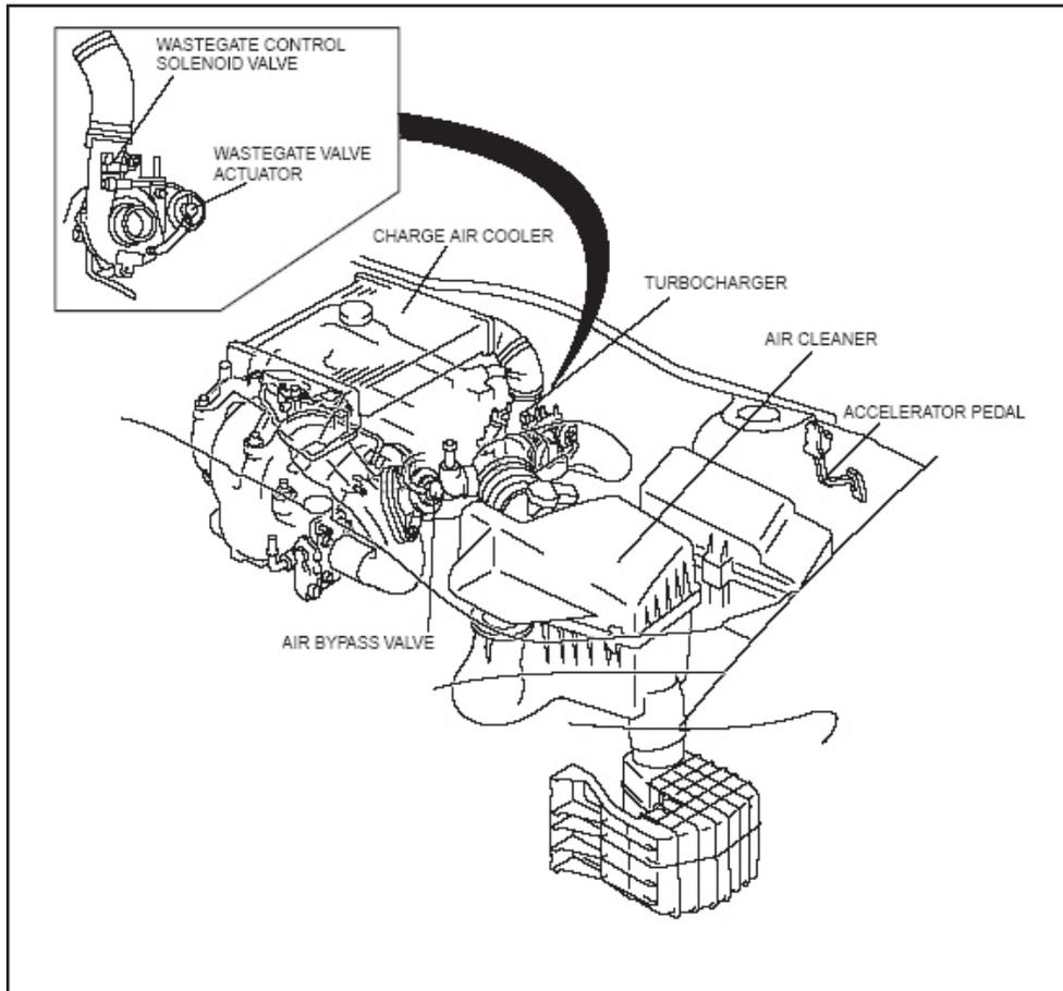
The main components of the turbocharging system are:
