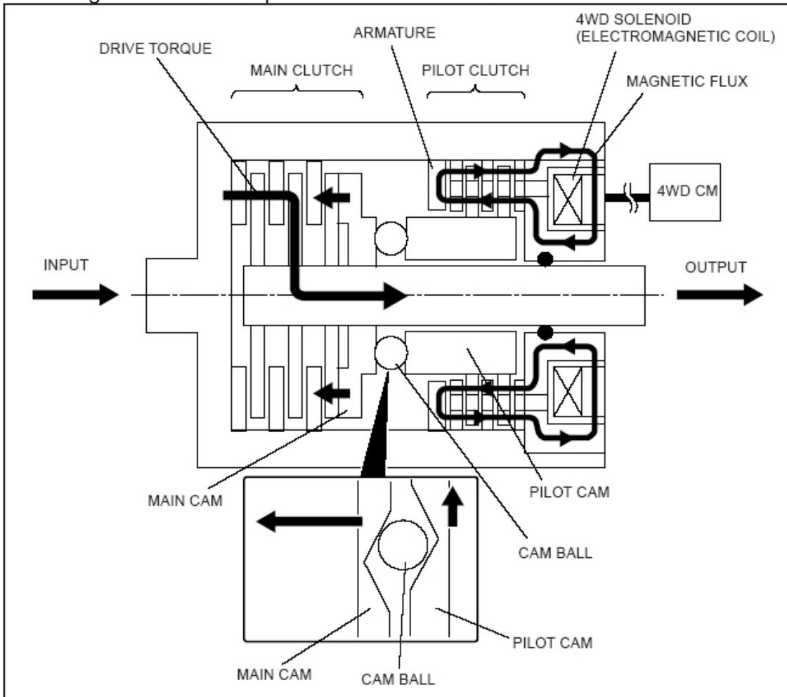
When the electromagnetic coil is energized and the front wheels rotate at a different rate than the rear wheels, the ball separates the main cam and the pilot cam. This exerts force on the main clutch and torque is transmitted from the driveshaft to the rear differential.
