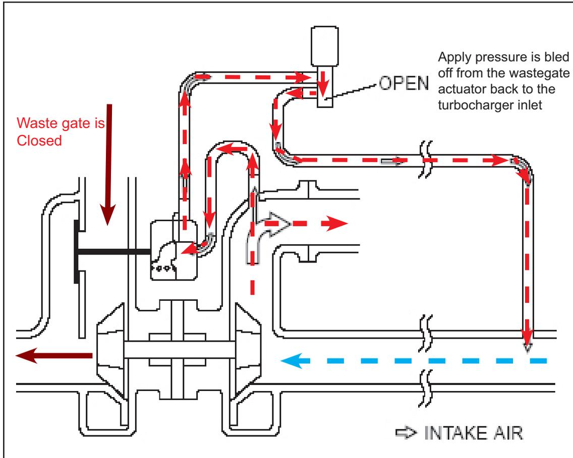
The waste gate regulator solenoid tunes the opening rate of the waste gate to help build maximum boost when needed. The solenoid controls the line from the intake manifold to the waste gate actuator. When the solenoid is energized, it bleeds off pressure routed from the intake manifold to the waste gate actuator. The solenoid bleeds this pressure back into the turbocharger inlet.
