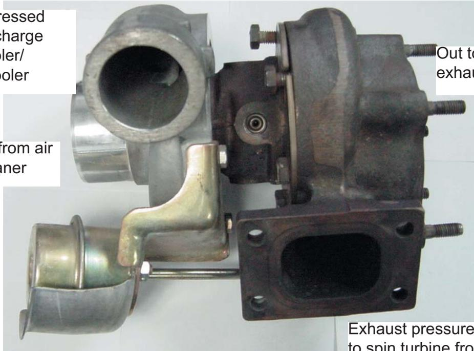
Exhaust pressure to spin turbine from exhaust manifold
