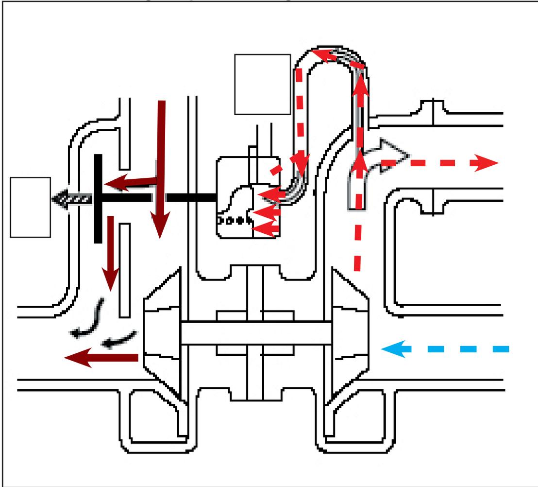
When boost pressure is high in the intake, the boost pressure from the intake manifold acts on the waste gate actuator to open the waste gate, slow down the turbine, and prevent an over-boost condition.
