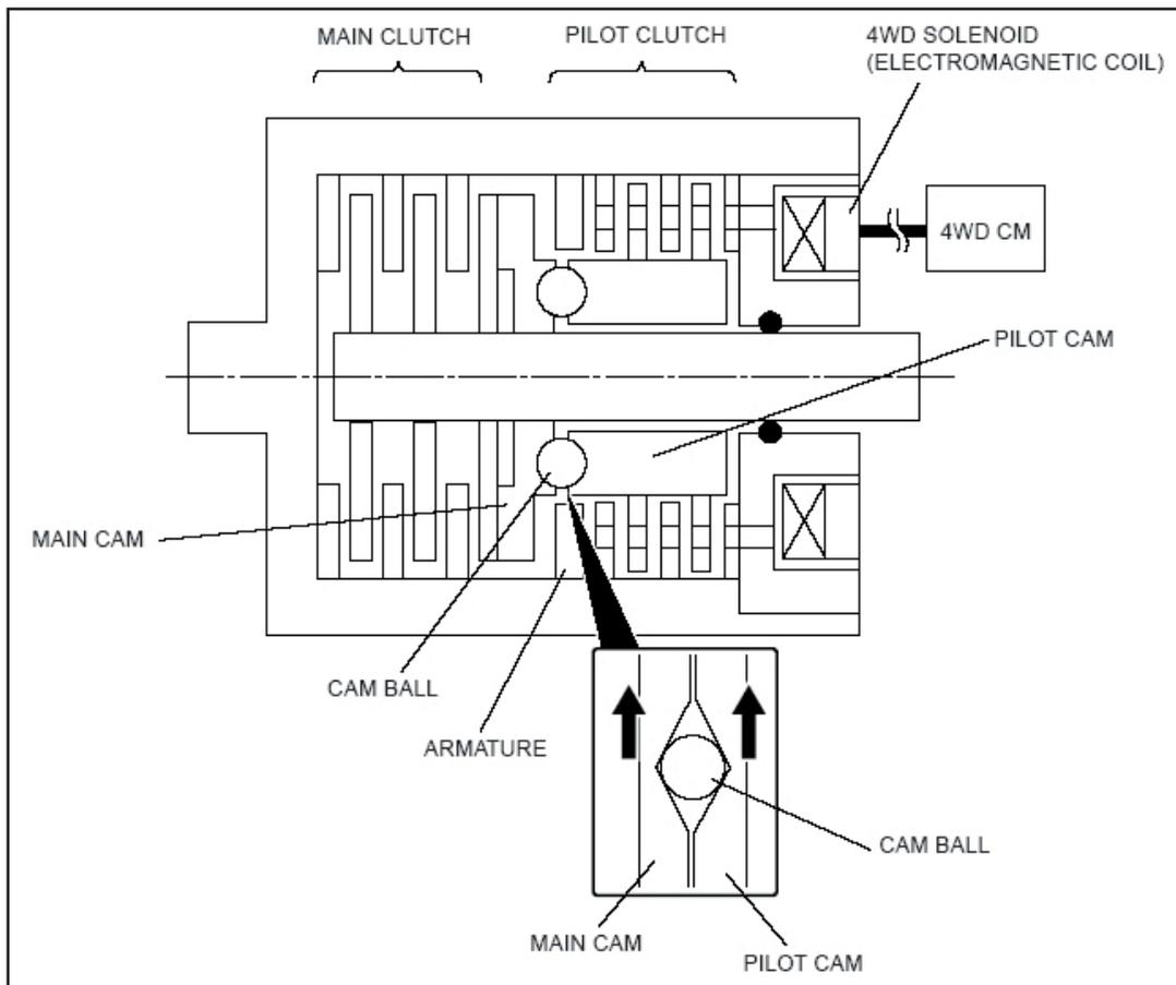
The ball is centered in the pilot cam so no pressure is exerted on the main clutch and no torque is transmitted to the rear differential.
